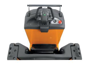
The combined lift of the control column operator platform up to 1,200 mm from the ground (model 620 PM-T ac) allows reaching a picking height of up to 2,800 mm.
