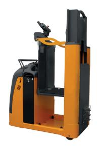
The buttons for slow forward/reverse, backing (optional), are located on both sides of the backrest and are useful for carrying out horizontal movements without climbing back inside the machine.
